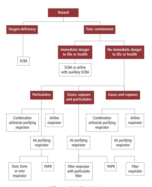
PAPR = powered air purifying respirator SCBA = self-contained breathing apparatus
